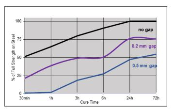
Fixture time and cure speed achieved as a result of using **ReAct**® **730** depend on the activator used, the substrate bonded, surface cleanliness and whether one or two surface activation is used.
