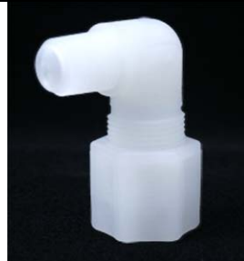
1/8" NPT X 1/4" Tube X 90° Kynar Fitting
