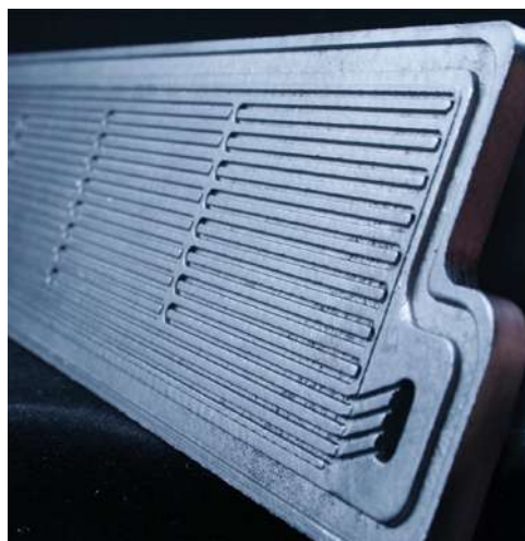
A graphite plate impregnated with GPS
